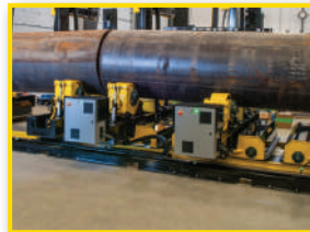
Sections brought together using powered track drive.
