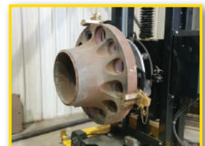
Optional Tailstock system available for adding flanges or end caps.
