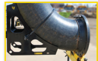
Fasten elbow into the jig.
