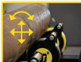
Alignment, side shift, and leveling functionality.
