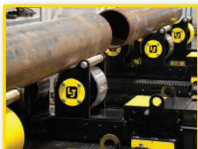
Pipe loaded, lined up using track drive.
