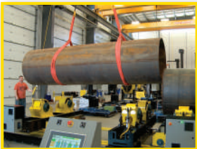
Each section loaded onto rolls.
